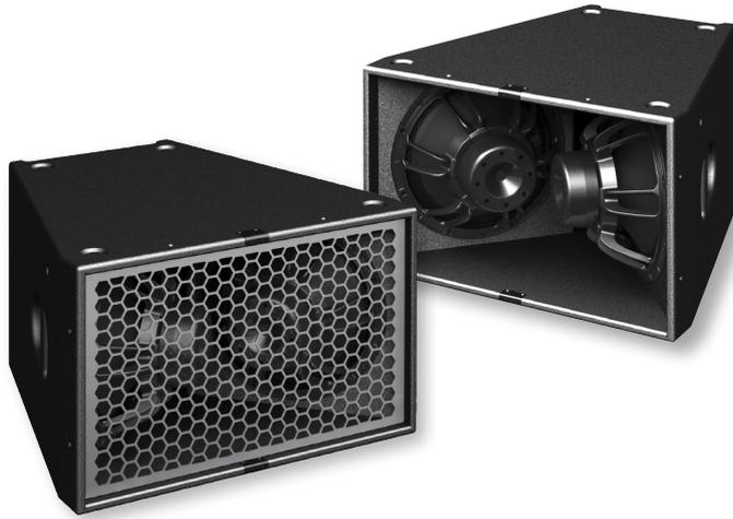
The PS 1 EX extension module doubles the performance of the PS 1 system in the 80 Hz to 300 Hz range (6 dB more sound pressure level). This provides noticeably more punch and dynamics for larger events and open airs. The two 12-inch drivers can be driven via the same amplifier channel as the low-mid path of the PS 1; all that is needed is a customised preset that takes the additional sensitivity into account.
