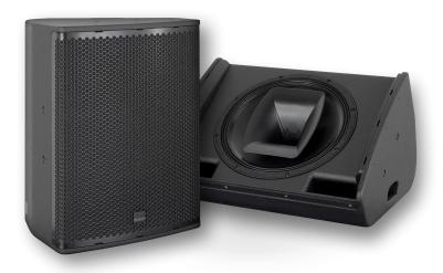
Multifunctional premium-class compact 2-way system. The coaxial configuration in combination with a carefully designed large-area horn ensures absolutely constant response even off the main axis. High-power Neodym drivers and long-excursion coils provide high efficiency and reduced distortion. Nine M10 threaded mounting points are available to mount MultiRigg hardware and other accessories for installation or mobile applications.
