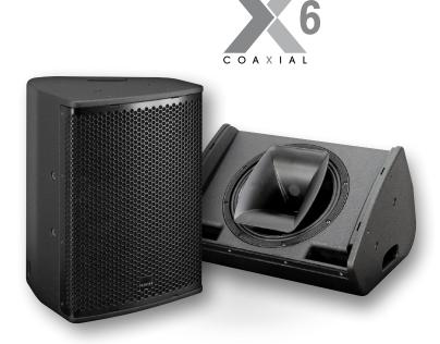
Multifunctional premium-class compact 2-way system. The coaxial configuration in combination with a carefully designed large-area horn ensures absolutely constant response even off the main axis. High-power Neodym drivers and long-excursion coils provide high efficiency and reduced distortion. Nine M10 threaded mounting points are available to mount Multi-Rigg hardware and other accessories for installation or mobile applications.
