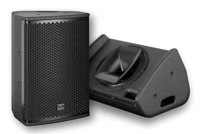
Multifunctional premium-class compact 2-way system. The coaxial configuration in combination with a carefully designed large-area horn ensures absolutely constant response even off the main axis. High-power Neodym drivers and long-excursion coils provide high efficiency and reduced distortion. Nine M10 threaded mounting points are available to mount MultiRigg hardware and other accessories for installation or mobile applications.
