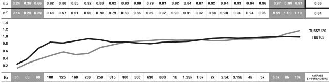
■ ABSORPTION COEFFICIENT: Values in accordance with the standards: EN 20654, ASTM C423 and EN 11654.
